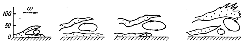
Fig. 7. Formation of vortices and ejections in the zone near the wall (according to [49]).
